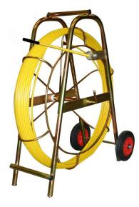
The Dart Systems Pipe Tracer (Flexitrace) provides a lightweight and compact solution for locating ducts, pipes and drains. The unit can easily be transported and deployed by one person and provides an alternative to traditional pipe location techniques using a Cobra Rod / Duct Rod and a Sonde Transmitter for the location of plastic pipes, pipe / duct obstructions or collapses.
