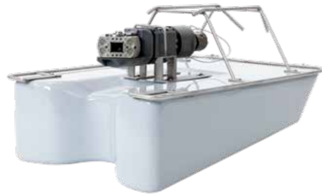
camera raft Application range from 600 mm for transporting a KS 135 through large water-bearing profiles.
