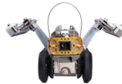
Attachment for egg shaped profile from 200/300 mm up to 900/1350 mm
