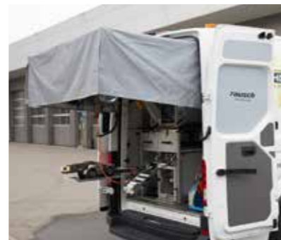
Folding rain and sun protection canopy
