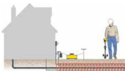
Direct connect to utility lines.
