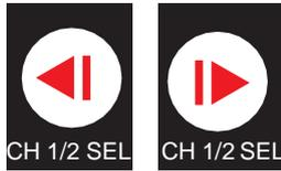
Whilst in 'Preview' mode, select the recording channel the camera is connected to by pressing either of the 'CH 1/2 SEL' (Channel Select) buttons.
