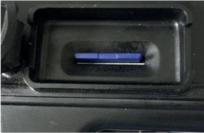
Insert SD card into Display Handset and replace cover to prevent water and dirt ingress.
