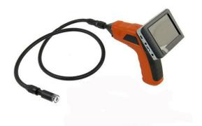
diameter and the cable is obedient which means it can be formed and will retain the formed shape. The unit is also supplied with a set of accessories including a Mirror, Magnet and hook which allow for pulling cables, retrieving lost keys / tools and side viewing.
