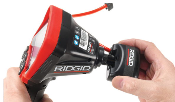
Figure 10 – Connecting the micro CA-300 Camera Monitor
