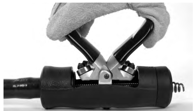
Figure 4 – Feeding Cable Through AUTOFEED
