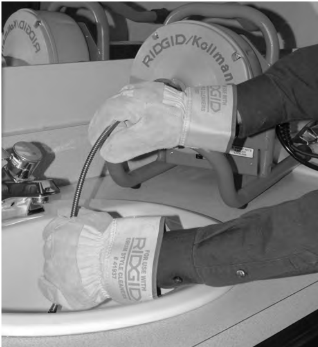
Figure 9 – Manually Feeding Cable
