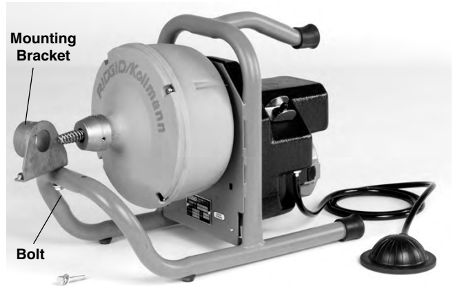
Figure 15 – Mounting Bracket Swung OPEN For Drum Access
