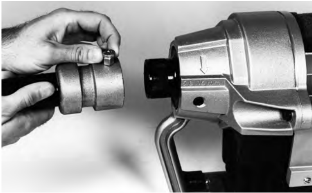
Figure 4 – Rear Guide Hose Attachment
