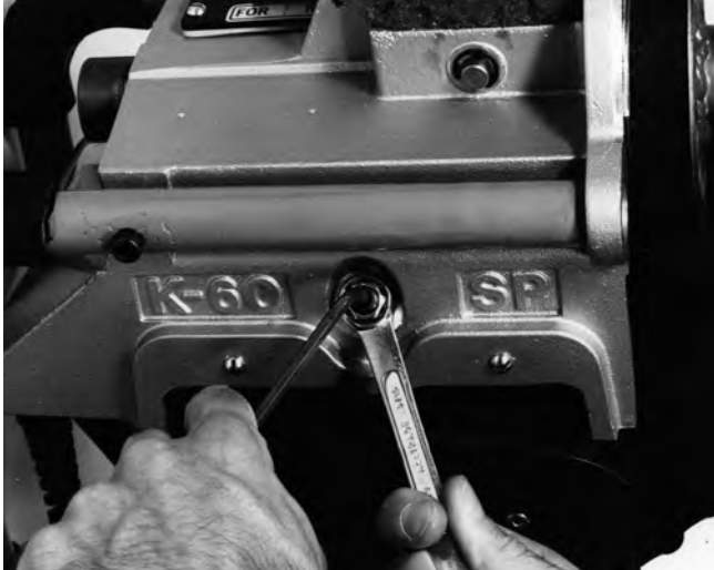
Figure 14 – Tighten Jam Nut
