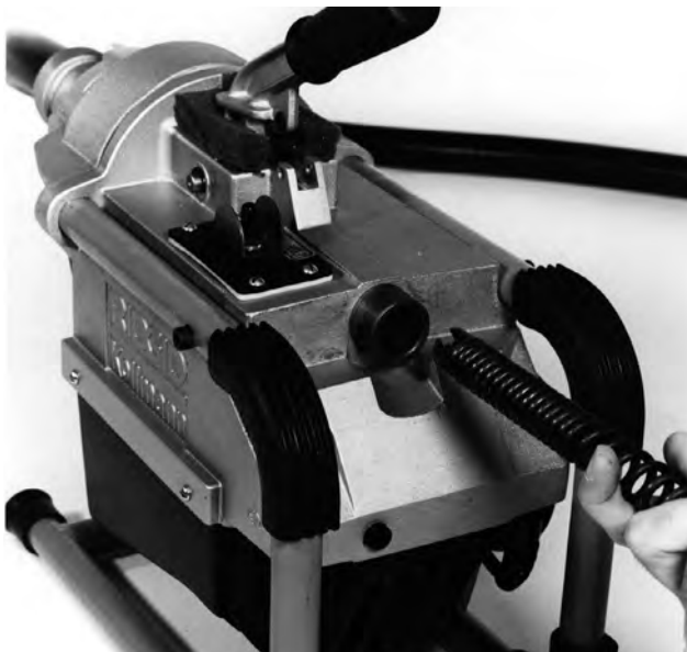
Figure 5 – Inserting Cable Into Front Of Machine
