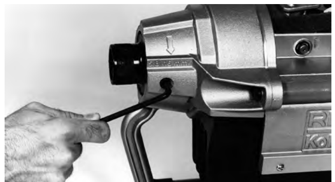
Figure 9 – Loosen the Set Screw
