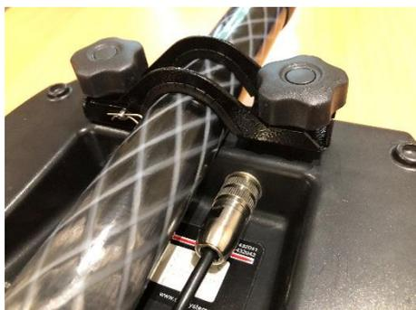
Attach the DS100 Monitor to the Camera Pole using the mounting bracket and star knobs provided. **Do not over-tighten.**
