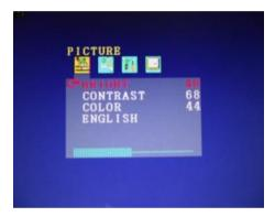
b. To flip screen imagePress Menu twice then Up/Down to select picture orientation.
